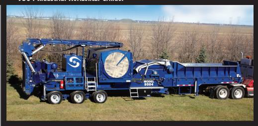
With a 40 x 60.5 inch feed opening and a CAT C27 1050hp Tier II diesel engine, this massive machine can grind an entire tree, branches or wood pallets. Equipped with an enclosed engine compartment producing the lowest decibel reading in its class and the only self-cleaning air intake system on the market, the 9564 is heavy duty and safe.
