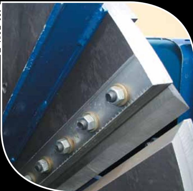
The chipping disc is 42" in diameter and 2" thick. There are four 7-3/4" knives in two locations on the disc. Four kickers help to discharge material from disc area. A convenient service lock pin holds the disc solid while servicing the knives on the disc.
