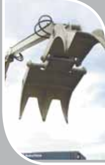
25' boom, continuous rotating grapple
