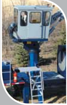
Cab raises 4' for unobstructed view of loading
