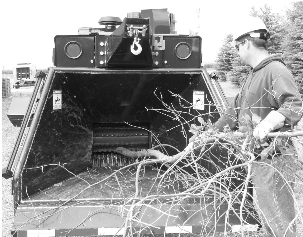
Figure 1.2 Proper position for feeding material into the hopper
