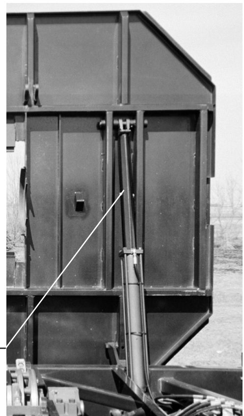
Safety stop in place on hydraulic cylinder
