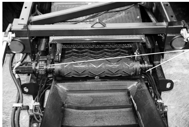
belly conveyor roller (Ref # 11)
